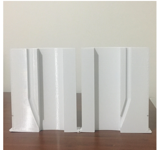
Figure 4.20: Aft strut as one piece (left), and parts separated (right)
