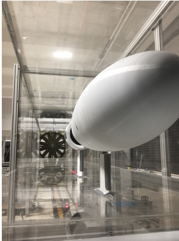
Figure 4.37: The front view of the BLI configuration
