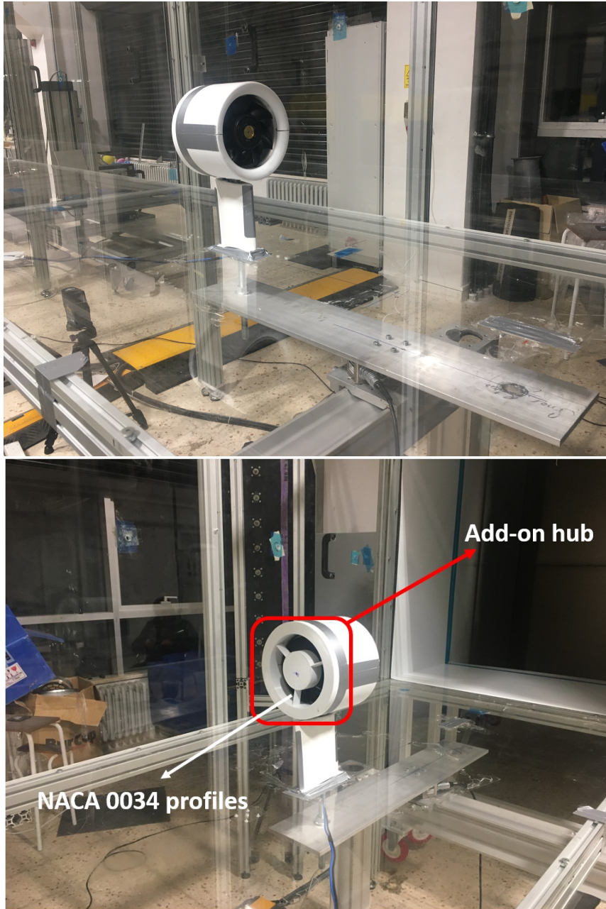
Figure 4.32: The overall look of the isolated propulsor configuration
